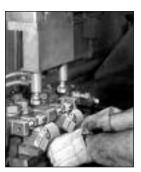
A Case History: Joining a piece of metal to itself is always tough. This job was done with an Equa-Press holder - two at a time.
