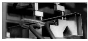
A Case History: Dual spot welding of panelled wall sections reduced welding costs enough to justify buying welding machine to do the job in-plant. Equa-Press holder with 5-inch spacing, and special (but simple) tooling to provide two offset tip adapters and matching holders were used. Electrodes are standard TUFFCAP caps.
